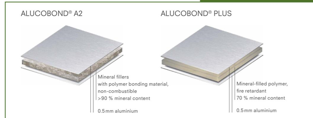
The composite structure of ALUCOBOND® consists of corrosion-resistant aluminium cover sheets. Aluminium is an excellent lightweight construction material which requires a high degree of primary energy during initial production, but is suitable for very long usage periods in the industry, transport and construction areas because of its optimum recycling properties (100 % infinitely recyclable).
