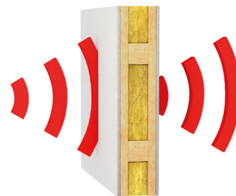
Wood, plaster walls. Loss: 5 to 20%
