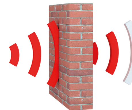
Brick, concrete. Loss: 20 to 40%
