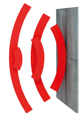
Enclosure in metal. Loss: 90 to 100%
