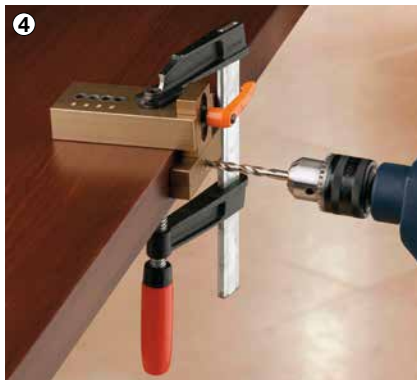
4 Drill Ø 7 mm guiding hole for stepped drill bit.
