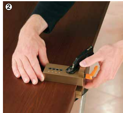
2 Flush door: Centre small drill plate on flush edge of door and tighten. Rebated door: Position small drill plate against rebate and tighten.
