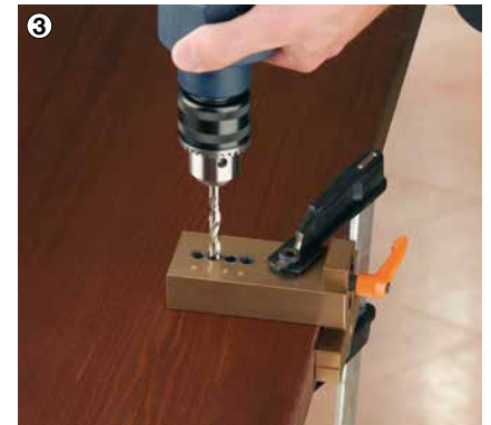
3 Drill Ø 7 mm guiding hole for HCS® hole saw.
