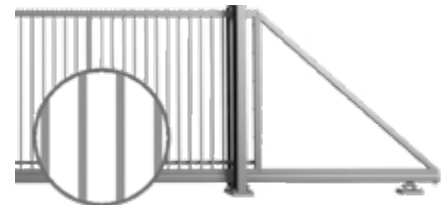
Closed box section infill 25x25mm [mm], CARO arrangement, welded to the structure.
