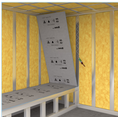
wedi Vapor 85 is direct bonded onto metal stud frames with the use of wedi 610 adhesive sealant...
