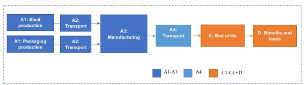
Steel and packaging materials are transported to a manufacturing plant where the stainless wall ties are manufactured. In this plant the steel is bent, cut and punched (all dry operations) to different shapes and sizes depending on which product that are manufactured. The wall ties are then distributed to the final customers. After use the product is transported to waste processing, and the steel is recycled.
