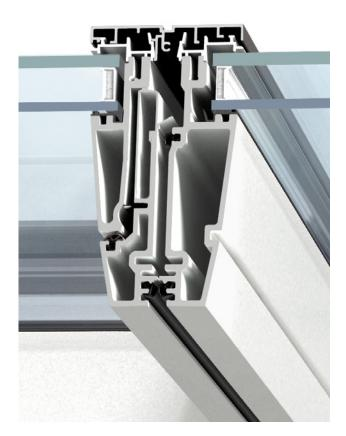
A two-level system with gaskets in the top and bottom ensures a very tight and durable connection between the two module profiles.
