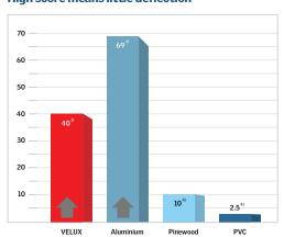
The high rigidity of the pultruded composite material makes the frame and sash extremely stiff. The rigid properties ensure reliable performance with very little deflection of the profiles and more durable aesthetics.
