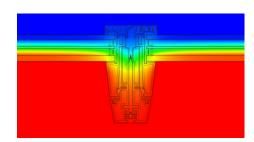
Thermal tests reveal the profile's ability to prevent cold bridging.
