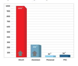
Compared to traditional skylight materials, the exceptional strength of the pultruded composite material allows longer and slimmer frame and sash profiles to be produced. As a result, large skylights with slim profiles become an option, which can lead to better aesthetic solutions.
