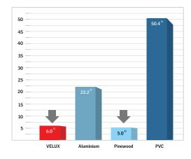
Traditional skylight materials fluctuate in form due to thermal changes, causing damage to gaskets and an increased risk of water ingress. Since the modular skylight composite contains 80% fibreglass, the profile properties are quite equal to those of the glazing unit. The similarity minimizes the risk of opposing movements in the construction, ensuring tightness of joints and a longer life expectancy of the application.
