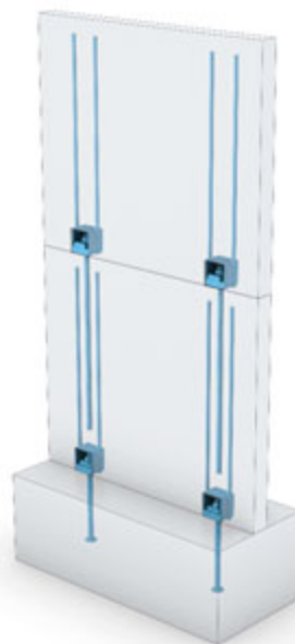
Figure 1. SUMO Wall Shoe and HPM, PPM Anchor Bolts in wall connection.
